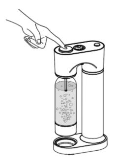
7. Press the exhaust button to release excess  $CO_2$  until the pressure gauge shows 0.
